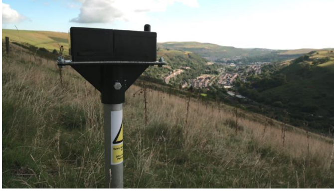
Figure 3: Tiltmeter sensor on a coal tip in the Rhondda Fach
