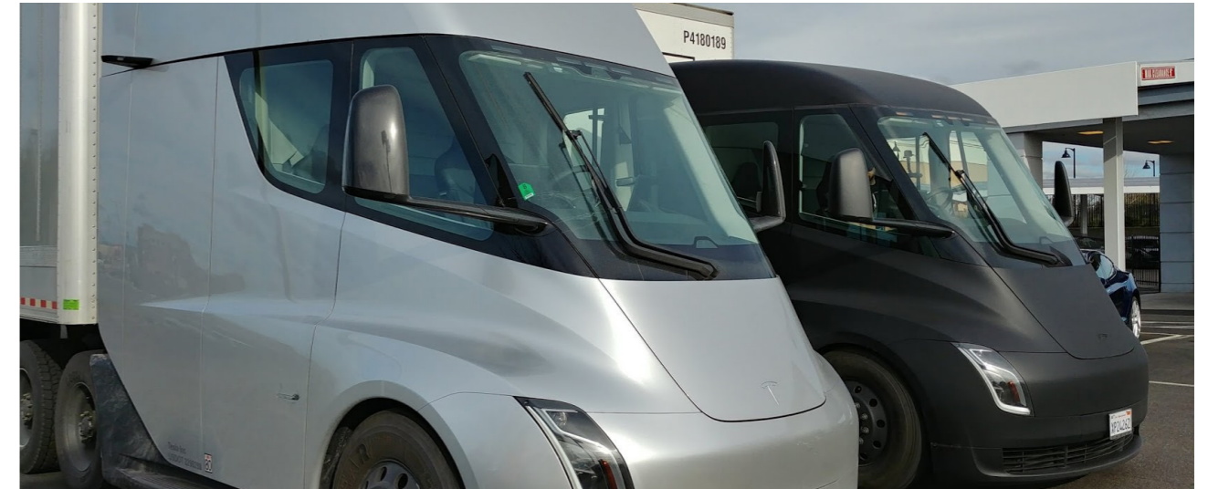
Figure 7 The Tesla Semi, a battery-powered HGV with a range of over 500 miles (taken by Korbitr, licensed under Creative Commons)
