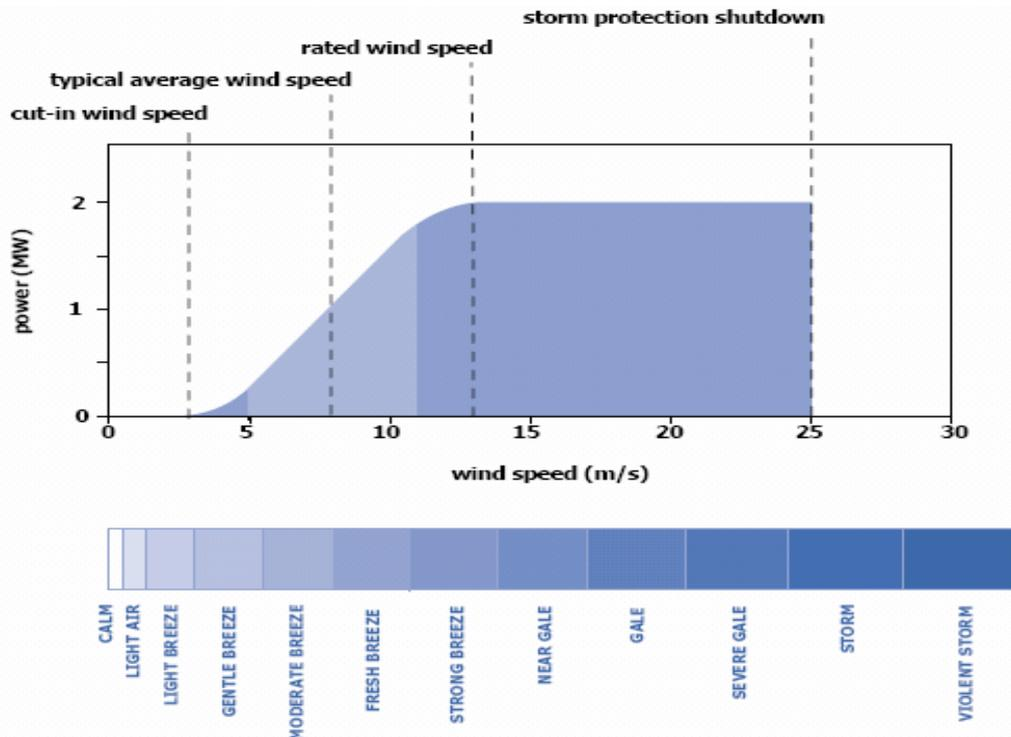
Figure 12 Typical power curve of a wind turbine. Source: BWEA<sup>144</sup>
