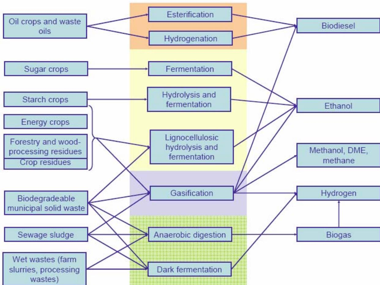
Figure 14 Feedstock, conversion processes and resultant products for biofuel production. Source: E4tech
